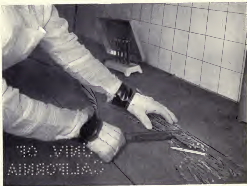
Chop the hardened Sticks with a pair of shears to the Desired Length
